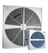
Rotary heat exchanger (wheel) is mainly used in building ventilation or in the air supply/discharge system of air conditioning equipment. The wheel transfers the energy (cold or heat) contained in exhaust air to the fresh air supplied to indoor. It's one important equipment and key technology in the field of construction energy-saving.
