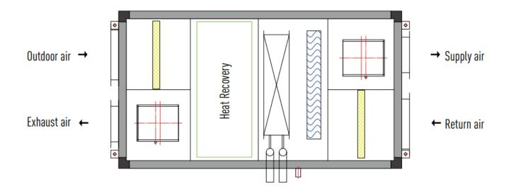
Type 4: Coarse and Medium Filter + Heat Recovery (with Bypass) + Heating/Cooling Coils + Humidifier + Fan
