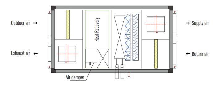
Type 3: Coarse and Medium Filters + Heat Recovery + Heating/Cooling Coils + Fan
