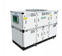
Package FAHU equipped with air to air heat exchanger plus DX coil before and after the air to air heat exchanger. Twice heat recovery to bring sufficient pre-cooling and heating the fresh air.
